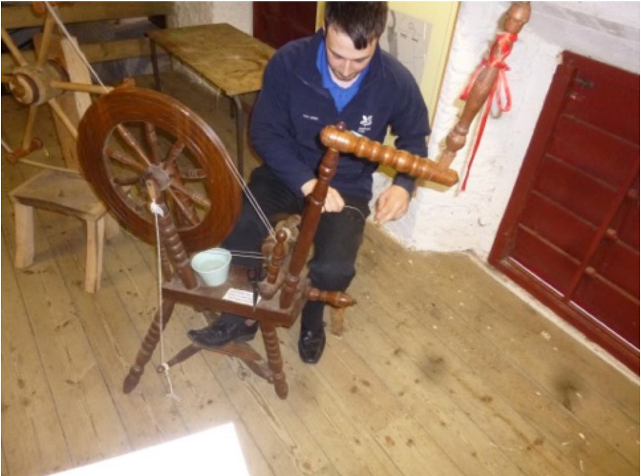
*Fairly standard spinning machine, note the cup of water to keep the fingers wet*
