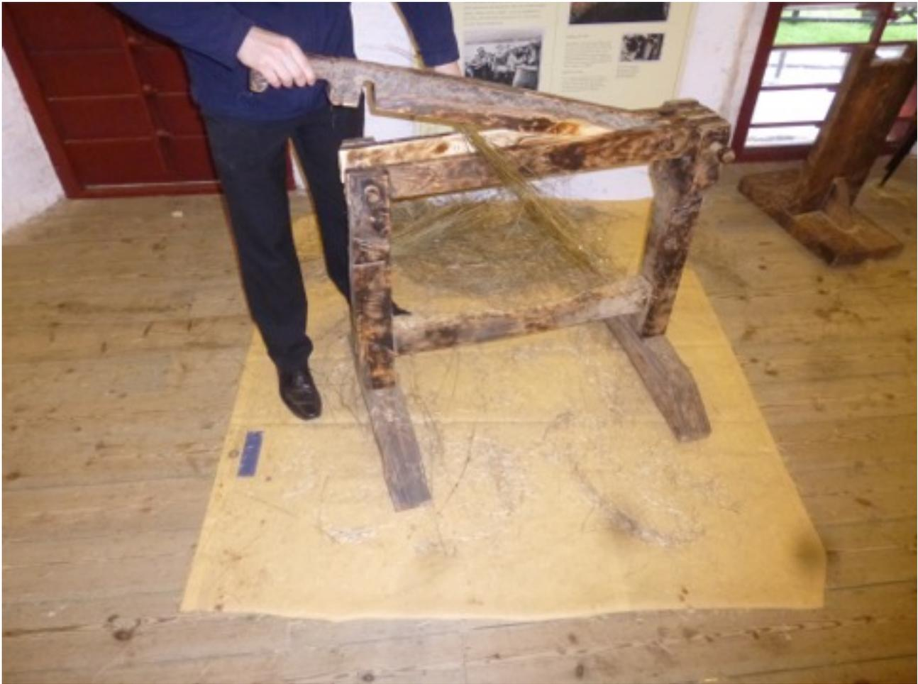
*Scutching, to remove the outer stem. SHOWS on the floor.*
