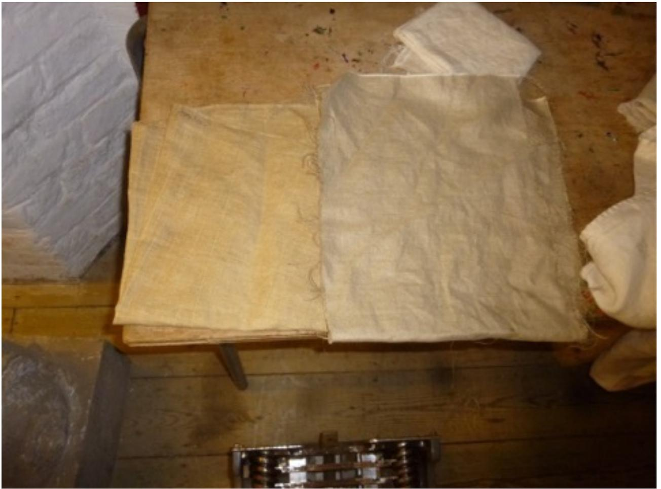
*The linen on the left after weaving, the linen on the right after beetling*
