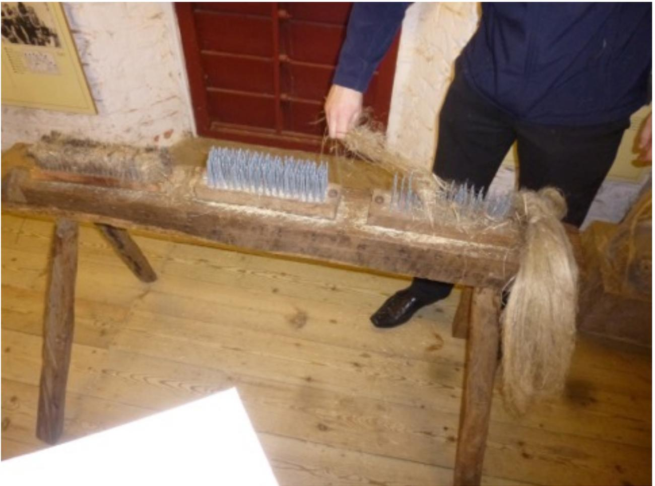
*Hackling or Heckling is the final process before the LINE appears*
